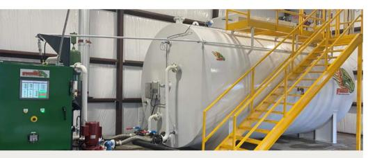
Greasezilla® is a turnkey standalone system that separates and processes FOG waste. The system's ecological grease-separating process removes FOG from the waste stream, reduces waste disposal expenses and creates new revenue. The system operates without dewatering, leaves nothing to be landfilled and has a total operating cost of 1-2 cents per gallon.
